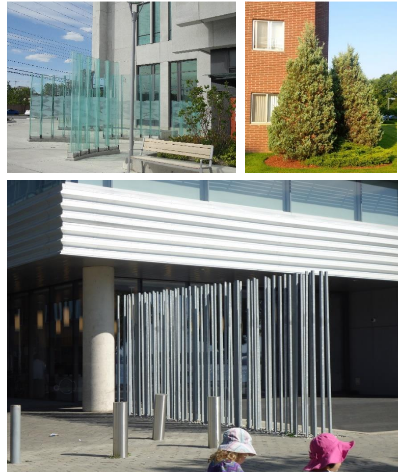
Image 11: Examples of Wind Mitigation Features around Building Corner
